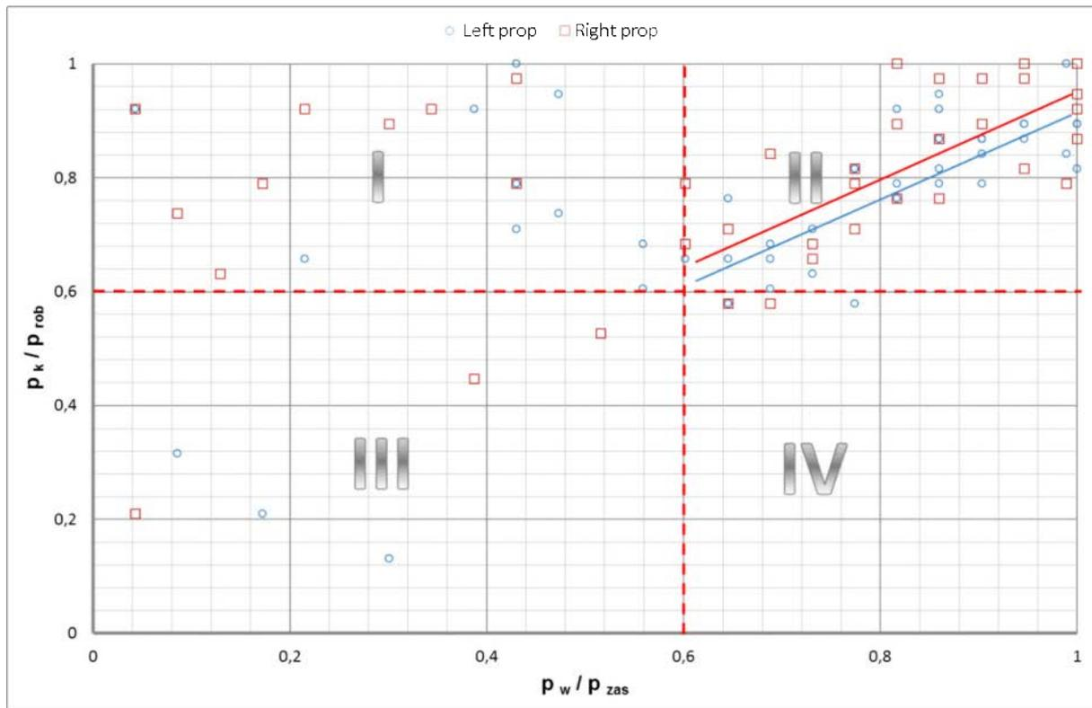
Fig. 7. Dependence of load bearing capacity on setting load  $p_k/p_{rob} = f(p_w/p_{zas})$  of props in powered support unit 72 for  $t_c = 120 \div 180min$  [3]
