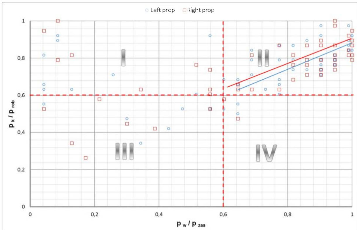
Fig. 6. Dependence of load bearing capacity on setting load  $p_k/p_{rob} = f(p_w/p_{zas})$  of props in powered support unit 72 for  $t_c = 60 \div 120 \text{ min}$  [3]
