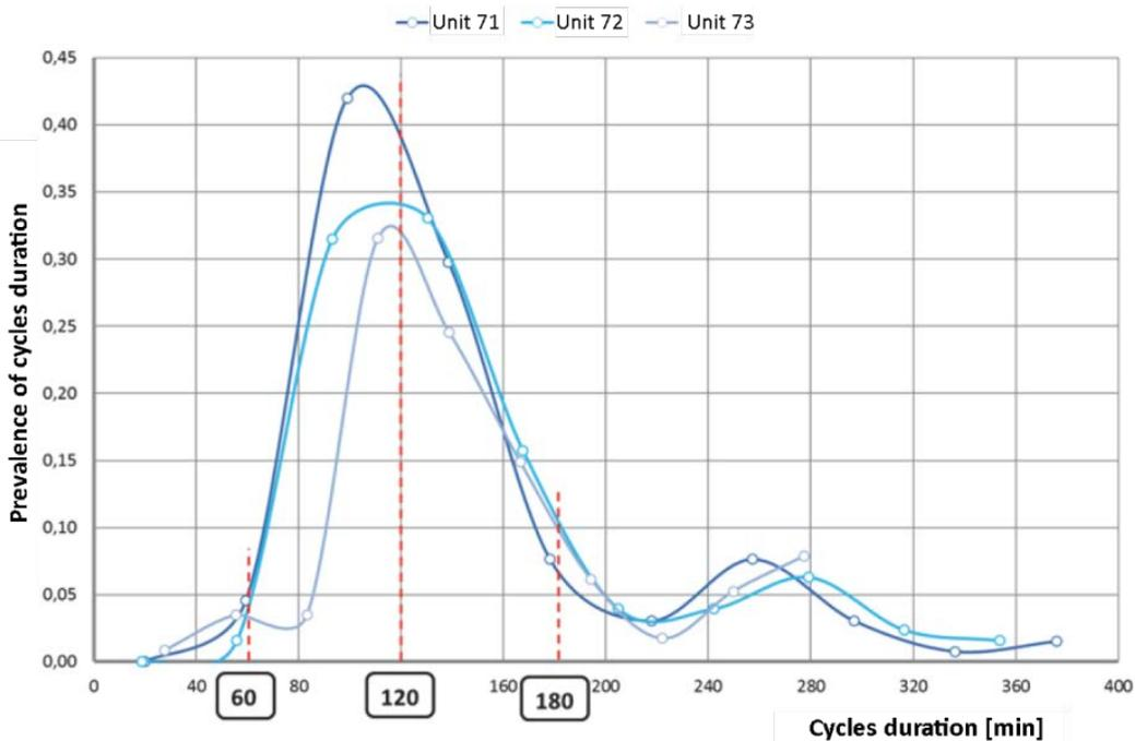
Fig. 5. Cycles duration  $t_c$  for three neighbouring units 71, 72 and 73 of the powered support unit [3]
