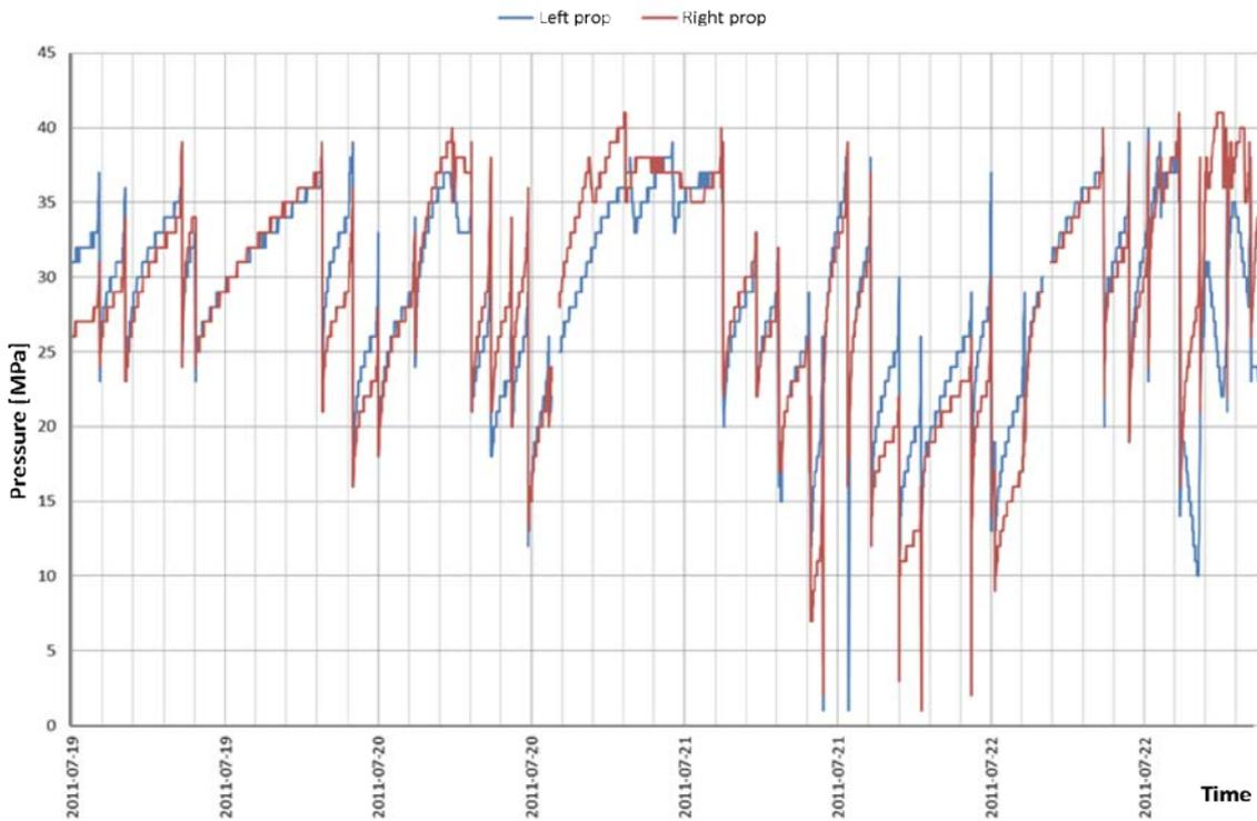
Fig. 2. Sample time series of pressure changes in under-piston compartment of props of the powered support unit during a few successive days [3]
