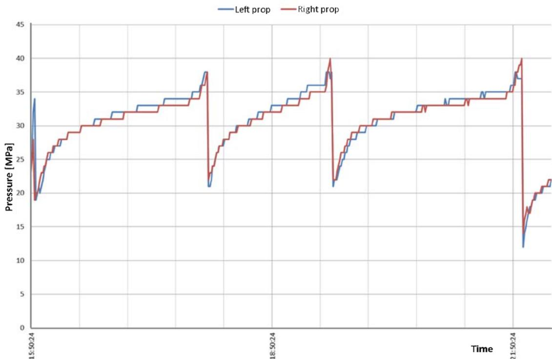
Fig. 3. Regular pressure increase in working areas of both props in the powered support unit [3]
