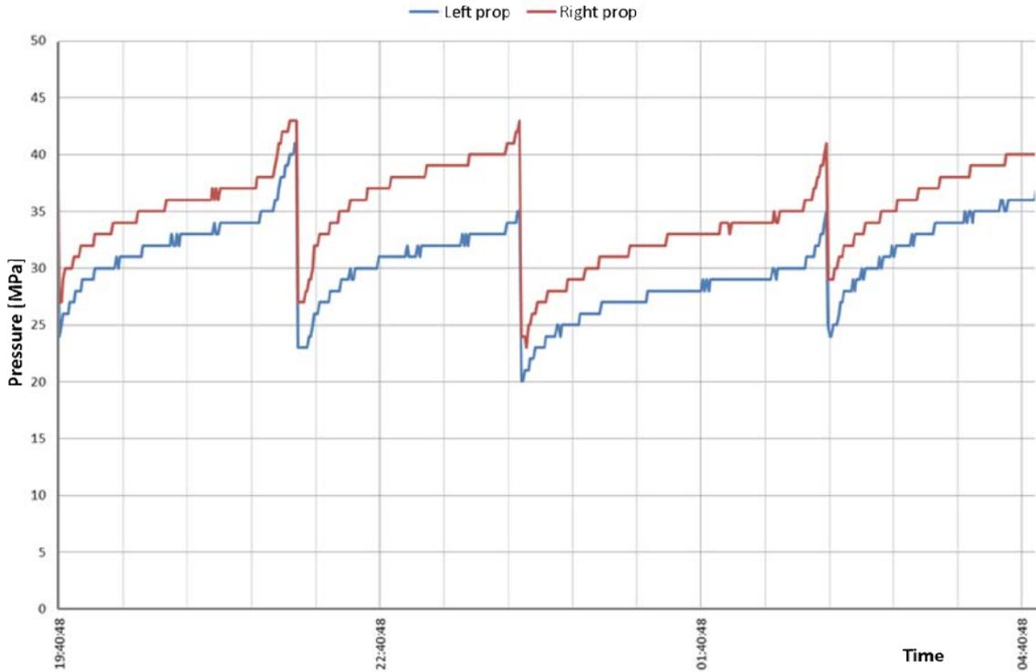
Fig. 4. Load cycles of the unit characterized by irregular setting of props [3]
